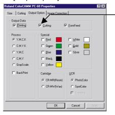
Make sure [Cutting] is selected when data includes the cutting data.
